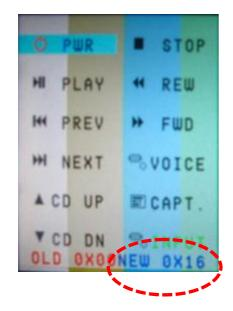
3. As soon as pressing the button, the remote button value displays at the right corner and it is saved automatically.
