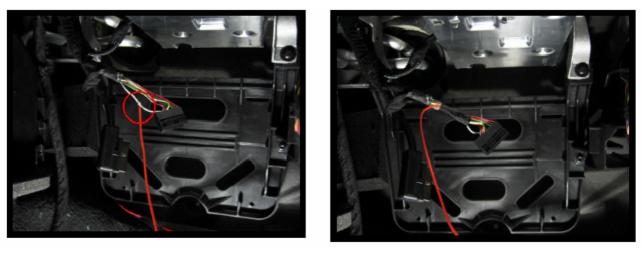
**③Connect Navi orange wire from Power cable to the 16<sup>th</sup> pin of the connector.**
