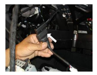
(9) Connect the offered LCD cable to OEM cable from LCD
