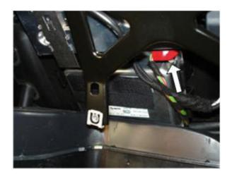
(6) Before installation, must unplug the red original Power plug.
