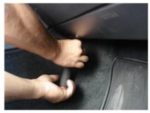
① Remove screws on Glove box.
