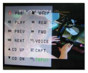
On AV1 mode, once touch the screen, Menu window appears like left picture. If no action for 5 sec or touch any other parts of the screen, this will disappear.
