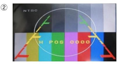
② After the setting done, rear parking guide line will appear in rear gear position. Once press "OK" button, "H\_POS" appears at the right and can adjust the line's position.
