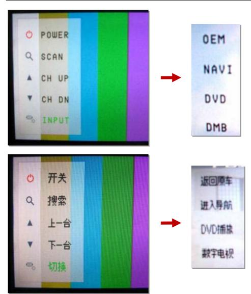
On AV2 mode, once touch the screen, Menu window appears like left picture. If no action for 5 sec or touch any other parts of the screen, this will disappear.
