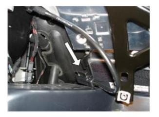
(8) Separate the cable from car.
