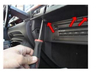
② Open Glove box after removing Screws on Dash board.
