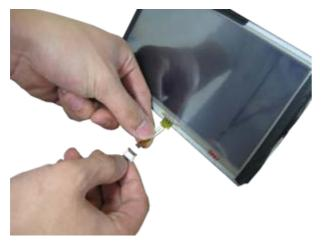
(1) Connect Touch Out cable to Touch from LCD
