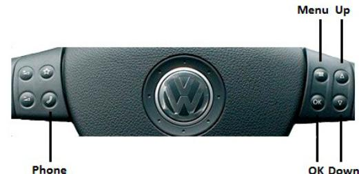
The music playback and settings are controlled from the radio, but it is also possible to select the next or the previous track from the steering wheel if Audio screen is selected on the cluster. The phone menu can be controlled from either the radio or the steering wheel (depending on the car and the radio specifications).
