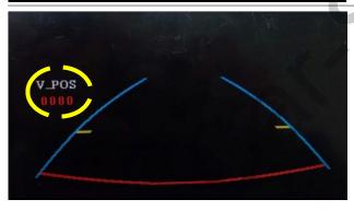
③ After adjusting horizontal position, press "OK" on the remote controller. Then you can see "V-POS" on the left of screen. At that time you can adjust vertical position of the guide line.
