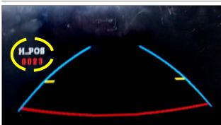
② If you get rear gear after setup, parking guide line will appear on screen as shown left. Now that you push "OK" button, you can see "H-POS" on the left of screen. Then adjust horizontal position of the guide line.
