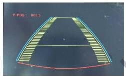
In V-POSITION use  $\triangle$ ,  $\bigtriangledown$  on remote control, to adjust parking guideline up and down.
