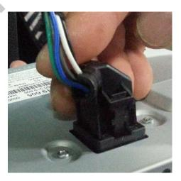
④ After The opposite connector of Provided "CAN IN/OUT" cable assemble the black plastic part, connect to behind of monitor
