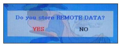
Step 5.) After all remote input finished, select "INPUT" on OSD, and press "OK" button of interface remote. Then, as left picture, confirmation window displays and ask confirmation.
