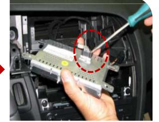
Remove the screws with a proper tool and monitor like the left picture.
