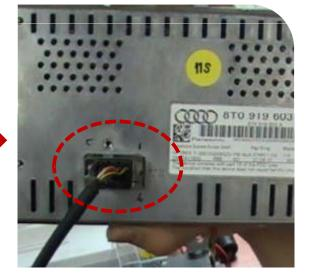
Connect the provided LCD-OUT cable between behind of LCD monitor and provided sub-board like left pictures.
