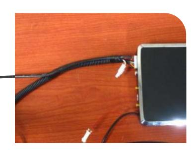
As the pictures, connect the provided Touch(NAVI) cable to "TOUCH(NAVI)" Connector of interface board and Navigation's Touch part.
