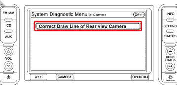
Image from the connected camera will be activated with OSD buttons for adjustment of parking lines and camera image. Align parking lines relative to the center of the image and adjust the lines accordingly.
